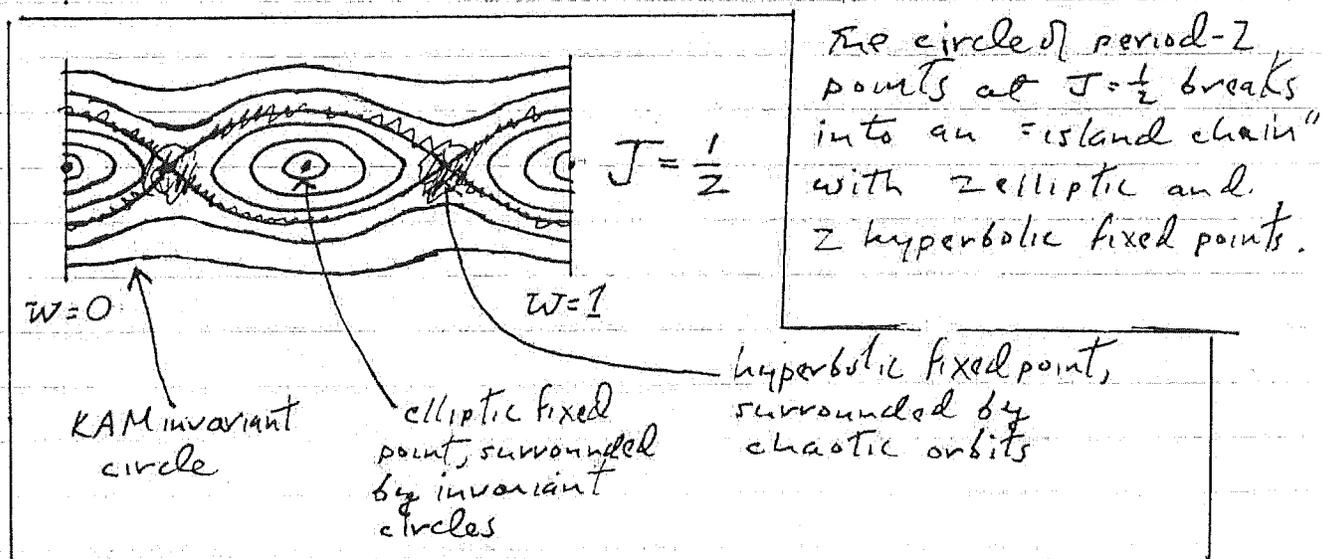
orbits are chaotic near the hyperbolic fixed points. Elliptical fixed points are surrounded by irrational invariant circles. The rational circles around the elliptical fixed points, upon closer inspection, break into still smaller island chains, etc. ...
