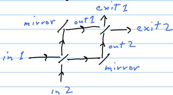
We can build an interferometer by combining two beam splitters and two mirrors as shown, where both beam splitters realize the unitary matrix  $\hat{U}$ .
