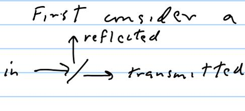
We can describe how the beam splitter acts on a single incident photon using a unitary  $2 \times 2$  matrix. The photon can enter the beam splitter via either one of two input "ports"
