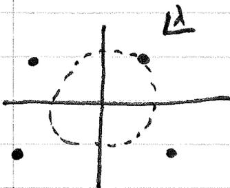
The radius of convergence of an expansion about  $\lambda=0$  is determined by the closest singularity of  $(1 - \lambda K)^{-1}$  to the origin.
