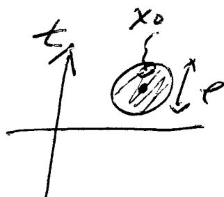
The action density is localized in a region in Euclidean spacetime with center  $x_0$  and radius of order  $\rho$ . It is because the action density is localized in time as well as space that this object is called an "instanton" (or "pseudoparticle")
