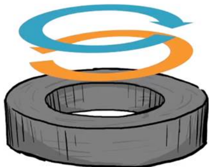
Persistent current in a superconducting circuit
